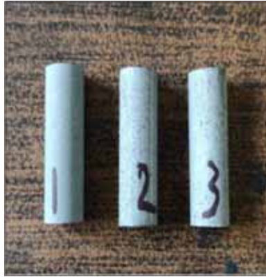
Fig. 3. Wear test specimen.
