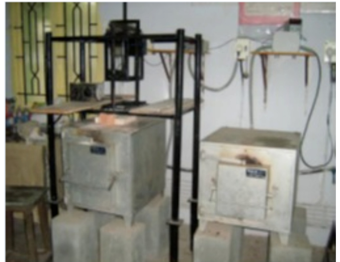
Fig. 3. Fabrication of LM6 alloy using stir casting setup.
