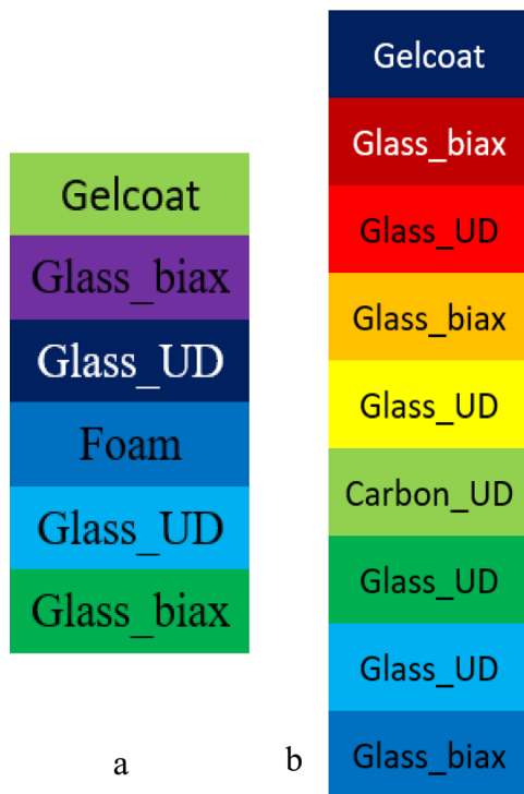
Fig. 6. Composite stack-up (a) fillers including LE_SS_filler, LE_PS_filler, TE_SS_filler and TE_PS_filler. Glass_UD: unidirectional glass fibre, Glass_biax: biaxial glass fibre, Gelcoat: coating for UV protection. (b) Spar_SS and Spar_PS. Carbon_UD: unidirectional carbon fibre.
