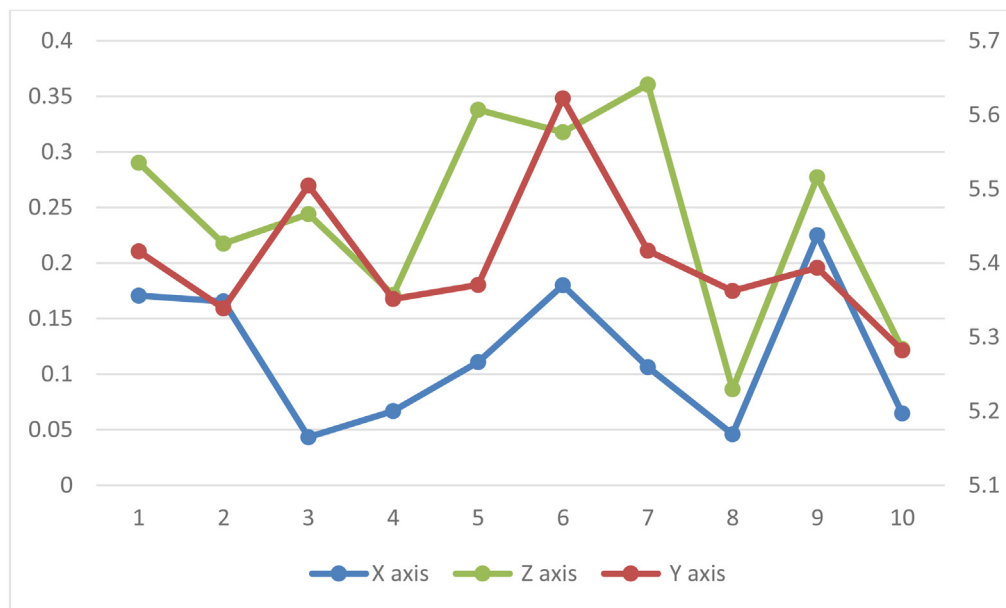
Fig. 22. Orientation of fixture about three axes in degrees determined by CBPEM using capacitance drop-based contact detection, angles in degrees for X- and Z- axis on left vertical axis with Y-axis pose in degrees on right vertical axis, and instances on horizontal axis.
